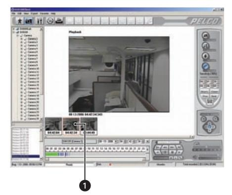
Figure 72. Thumbnail Images Marking Pixel Changes
